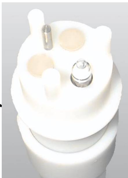
Bottom view of electrode holder with one electrode installed and potential matching pin
